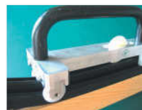
notching of the continuous gasket
